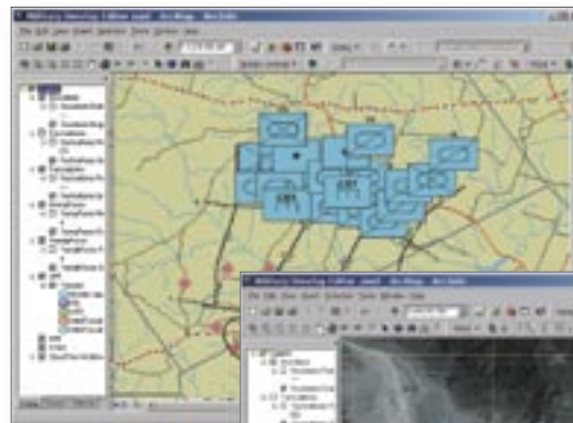
The Geodesy Tools provide analytical tools for calculating great circle routes, rhumb lines, lines of bearing, and range rings used in geospatial analysis for military planning.
