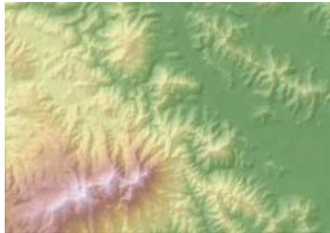
This map shows elevation combined with hillshading. The combination of these display methods creates an attractive map that simultaneously shows heights and the surface shape.
