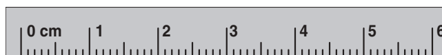
In this example, the ruler represents a hatch class. The interval of the hatches is 0.1 cm (1 mm). There are three hatch definitions. Each definition is placed at a multiple of the hatch interval—10, 5, and 1, respectively. Some hatch definitions are labeled, while others are not.
