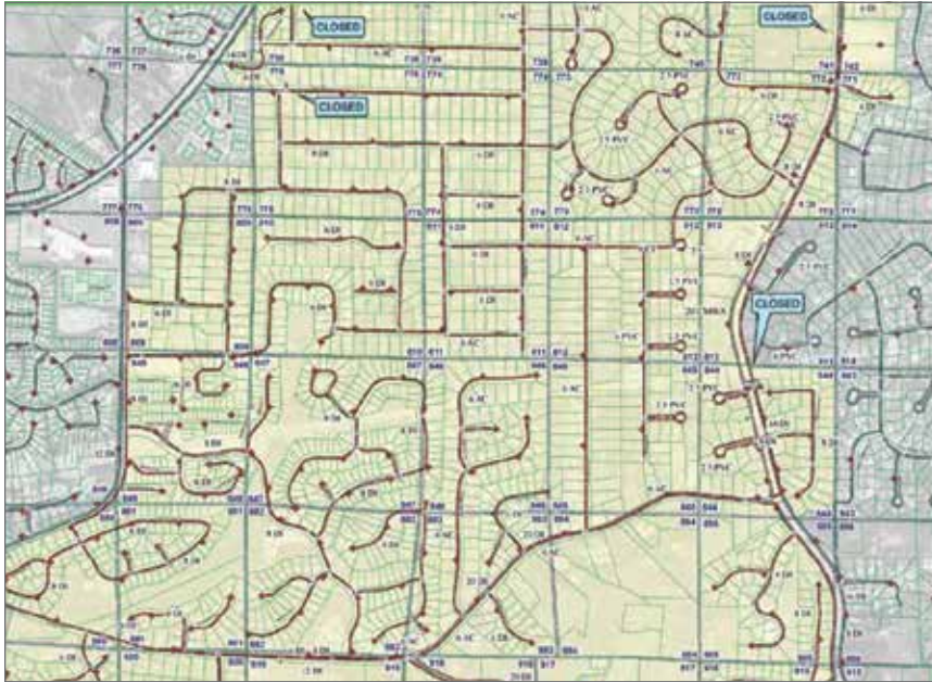
This utility map shows parcel locations, water lines, and valves for Cobb County Water System in Marietta, GA. Map courtesy of Cobb County Water System.
