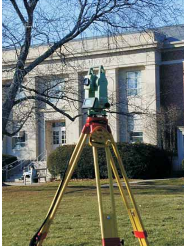
Figure 1.1: A total station is a theodolite and an electromagnetic distance measurement (EDM) instrument packaged together.
